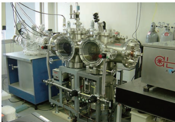
Figure 1 Photograph of the atomic oxygen beam facility used in this study. Two 1500 L/s turbo molecular pumps are used to maintain the vacuum.
