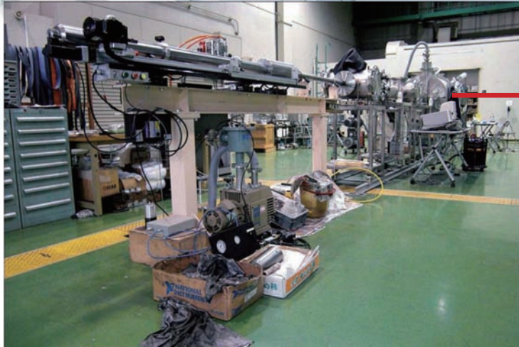
Two-stage light gas gun (ISAS/JAXA)
