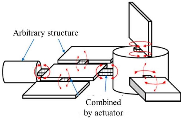
Fig. 1. Example of Transformable Structure of Spacecraft.
