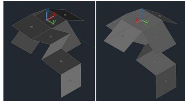
Fig. 8. The shape of spacecraft in case of best attitude stability
