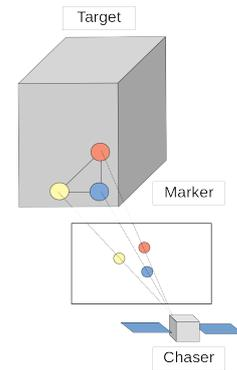
Fig.1 Image of a spacecraft that takes pictures of a target
