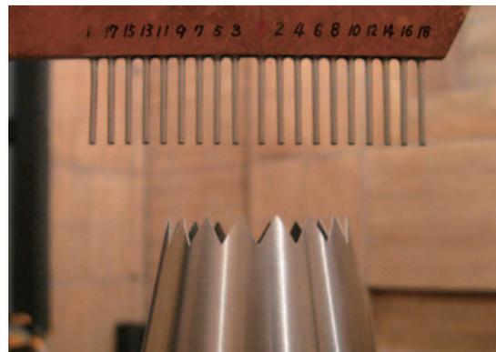
Fig.3B: A Rake used in Pressure Measurement.
