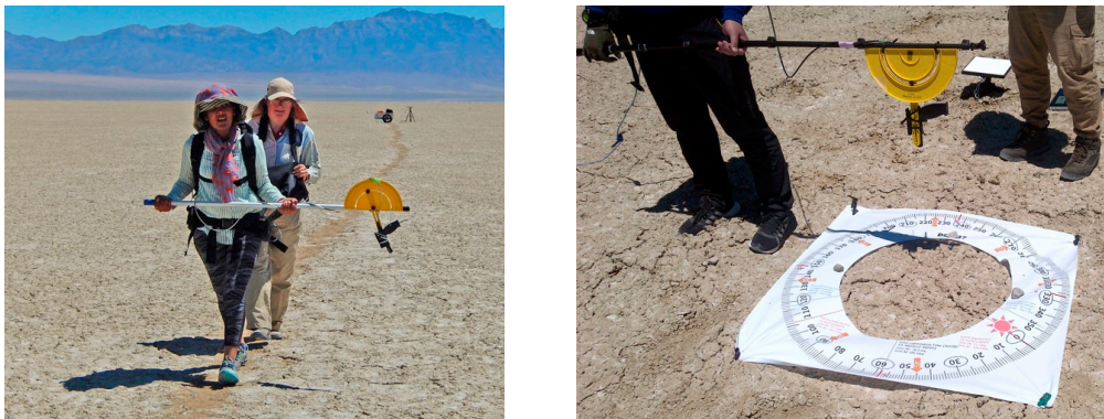
Figure 6. (Left) Protractor used to acquire off-nadir surface-reflectance data at Greenhouse gasses Observing SATellite (GOSAT) view angles; (Right) ground target used to identify view angles for off-nadir data collects.
