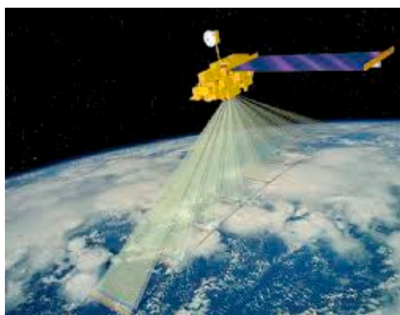
Figure 10. The Multi-angle Imaging SpectroRadiometer (MISR) instrument is one of five sensors on-board the Earth Observing System (EOS)/Terra spacecraft. Collecting data since early 2000, its radiometric response has been determined using VicCal campaigns.
