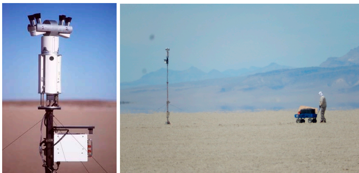
Figure 1. The Portable Apparatus for Rapid Acquisition of Bidirectional Observation of the Land and Atmosphere (PARABOLA) 8-channel hemispheric scanning radiometer. (Left) instrument closeup, where a Spectralon diffuse reflectance standard sits on top of the electronics module and is viewed during the nadir scan; (Right) instrument at a final height, with a field engineer for perspective.
