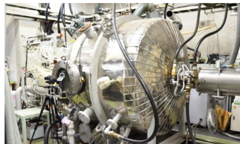
Fig.1 1MW arc-heated wind tunnel (ISAS/JAXA)
