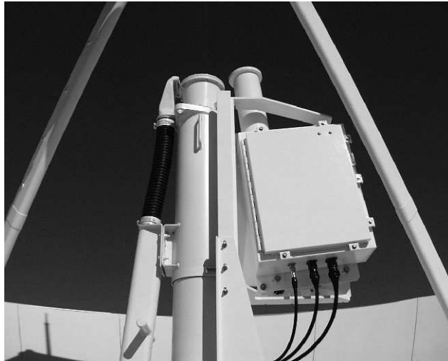
Figure 2: Radiometer mounted on the Usuda 10 m dish for tests. It was then unmounted to conduct further tests in the laboratory.
