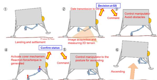
Fig.2. [One example of front loading activities] After studying an operational scenario on the surface of the Martian moon, a functional test of the robotic arm and corer mechanism was carried out to ensure satisfaction of the mission requirement: “To collect samples at a depth of two centimeters or more below the surface of the Martian moon.”
