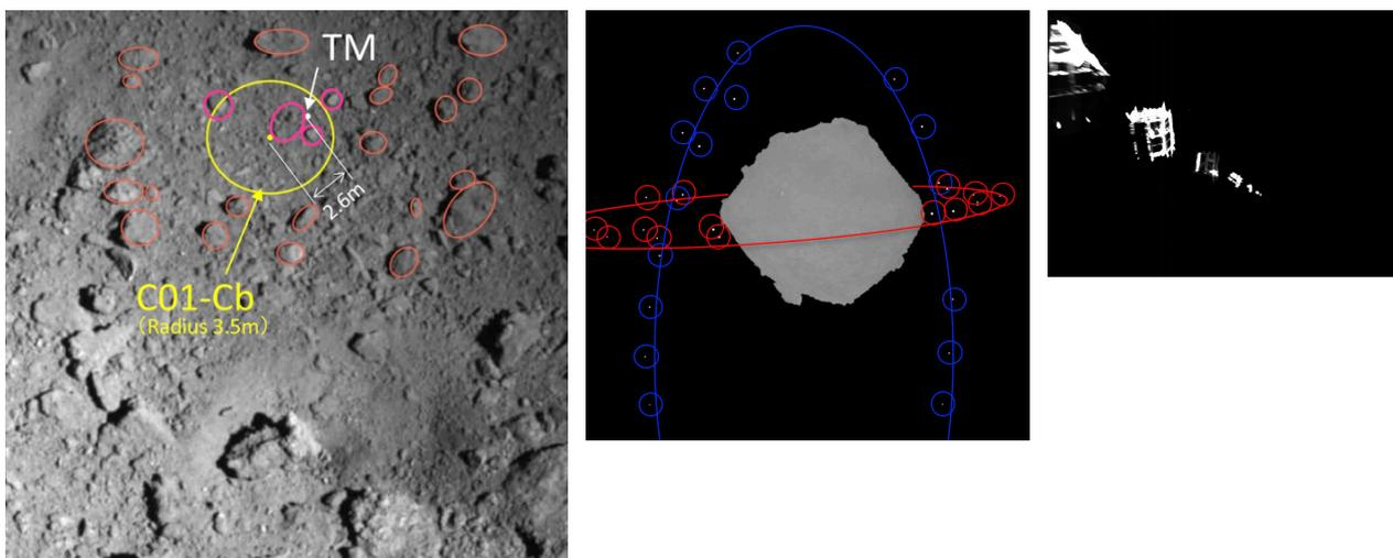
(Fig. 1. left) Artificial crater (bottom) and second touchdown point C01-Cb. The second touchdown point is an area with a diameter of 7m, about 20m away from the center of the artificial crater. The target marker was dropped onto the touchdown area. (© JAXA, University of Tokyo, Kochi University, Rikkyo University, Nagoya University, Chiba Institute of Technology, Meiji University, University of Aizu, AIST)
