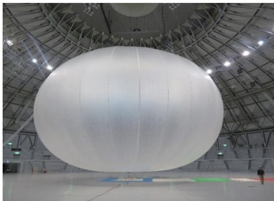
Fig.1. Fully inflated 6,400m<sup>3</sup> balloon.
