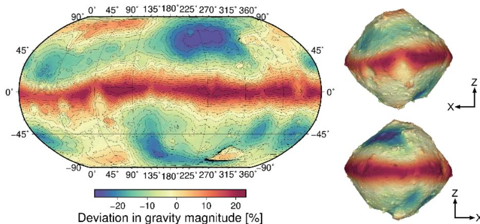
Fig. 1. Gravity field of the asteroid Ryugu. The deviation in the magnitude of surface gravity relative to the point-mass model.
