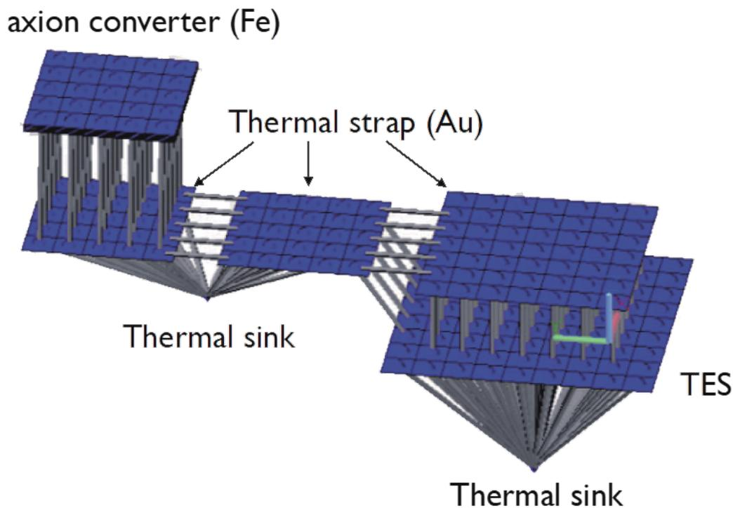
Schematic diagram of the TES microcalorimeter thermal FEM (Finite Element Method) model.
