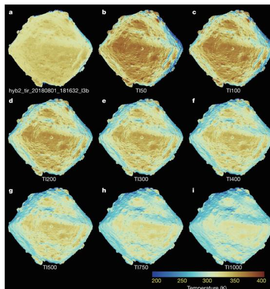
A thermal image of Ryugu taken on 1 August 2018 from a 5 km altitude in **a**, compared with calculated thermal images with uniform thermal inertia of 50 to 1000 tiu in **b-i**.
