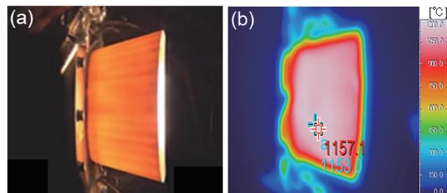
Fig. 3. Combustion test for a miniature-sized deployable nozzle: (a) optical camera image and (b) thermo-camera image.
