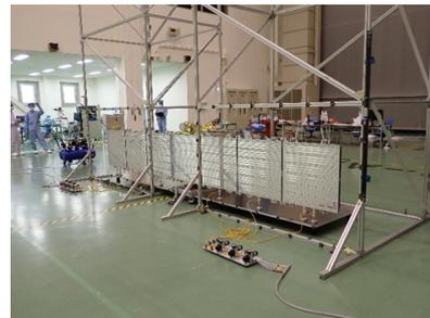
Fig.1. Deployable SAR Antenna
