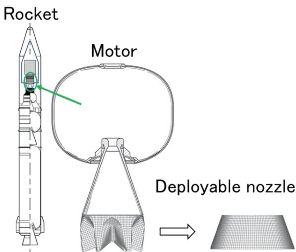
Fig. 1. Deployable nozzle extension for rocket motors.
