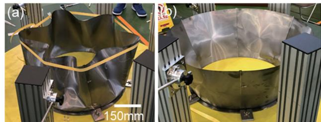
Fig. 2. Full-scale deployable nozzle (a) after folding with banding bands and (b) after deployment.
