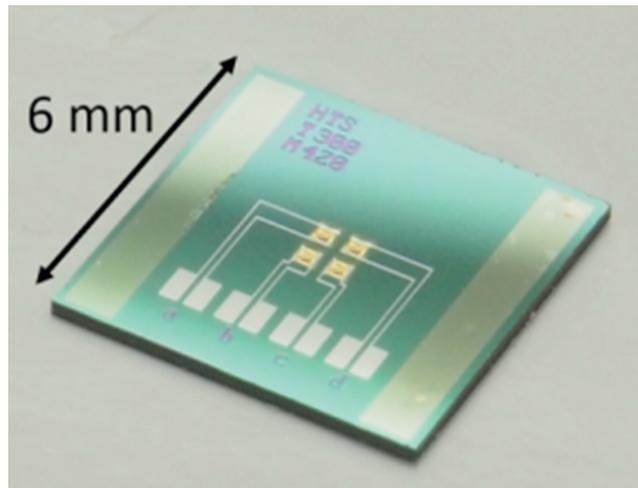
Picture of the TES detector, fabricated in-house at ISAS.
