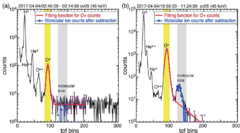
Time-of-Flight (TOF) spectral distributions of 45 keV ions observed by ARASE. (a) a 30-minute-integrated spectrum during the geomagnetically quiet time on April 4, 2017. (b) a 30-minute-integrated spectrum at the start of a small magnetic storm on the same day. Molecular ions, which are not seen before the onset of the magnetic storm, are detected during the magnetic storm.
