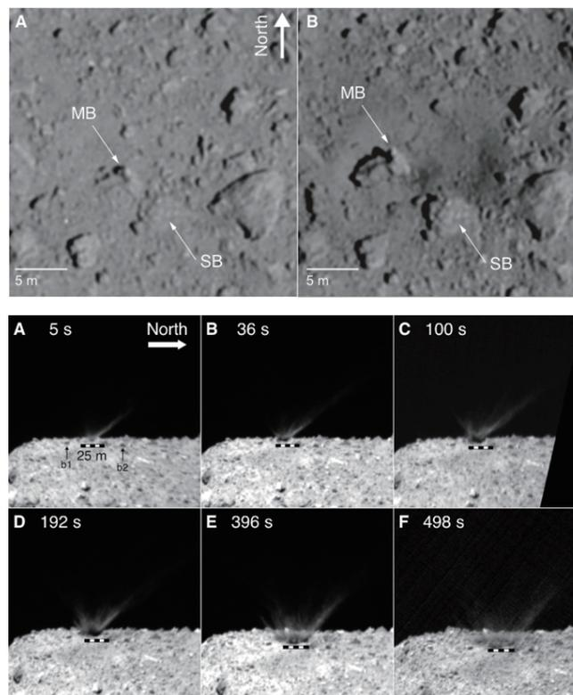
(above) ONC-T image. Ryugu surface before SCI operation (A), Artificial crater formed after operation (B). (below) DCAM3 image. Time difference from SCI operation is 5 seconds (A), 36 seconds (B), 100 seconds (C), 192 seconds (D), 396 seconds (E), 498 seconds (F). (M. Arakawa, *et al.* Science 2020)
