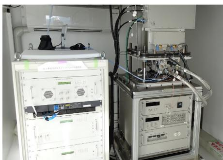
Receiving RF interface unit for Ka-band (left) and Low Noise Amplifier for Ka-band (right).
