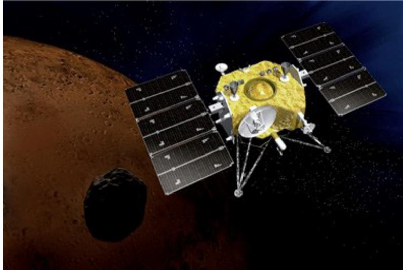
Fig.1. [Image of the MMX spacecraft] One possible MMX spacecraft configuration with a launch mass of 4,000 kg. The spacecraft consists of three main modules: return, exploration, and propulsion. The nominal mission duration will be 5 years.
