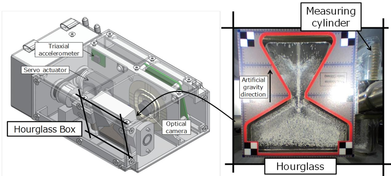
3D CAD Image of the Hourglass Box with hourglass and measuring cylinder (left) and the behavior of alumina beads in low gravity (right)
