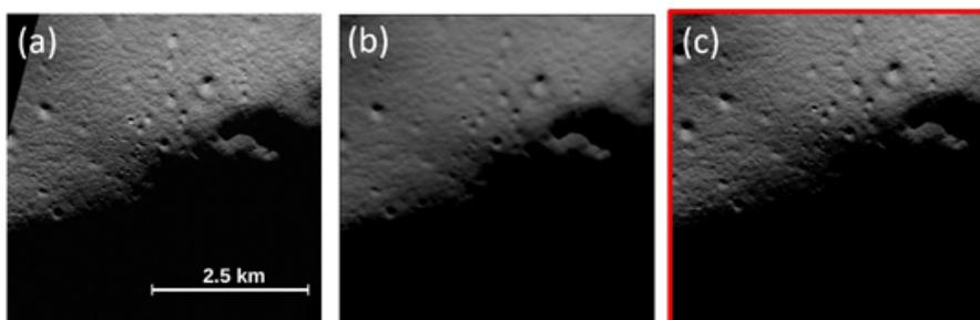
Our terrain model with improved accuracy. (a) Lunar Reconnaissance Orbiter (LRO) Narrow Angle Camera (NAC) image (50 cm/pixel), (b) conventional LRO Lunar Orbiter Laser Altimeter (LOLA) topographic model hillshade map (Glaser et al., 2014), (c) our terrain model hillshade map.
