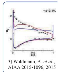
•  $C_{DES}=0.51$ ,  $C_{rot}=2.0$ , and Dirty-Cell Treatment ( $AR > 4$ ): Best Match with Experiment!
