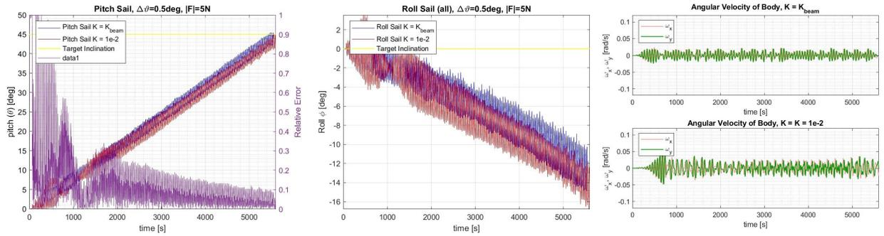
Fig. 3: Pitch (L), roll (C) and nutation of the probe (R) for  $K = K_{beam}$  and  $K = 1 \times 10^{-2}$  for tip-mass thrusting.
