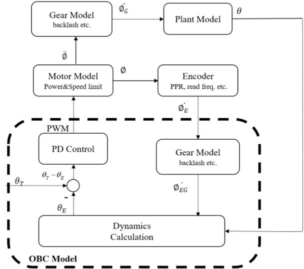
Figure 4 System diagram of the one-armed satellite simulation model
