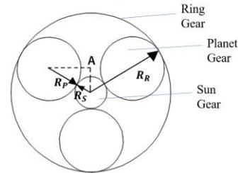
Figure 7 Planetary gear set sizes
