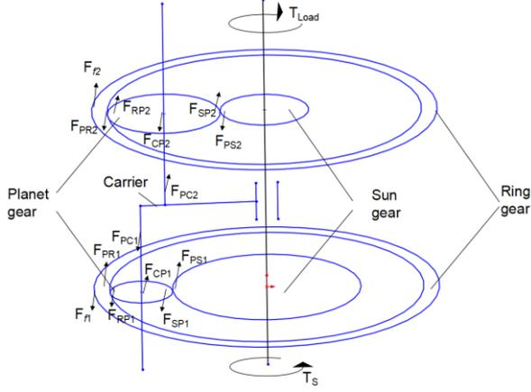
Figure 10 The diagram of 2-speed planetary gear transmission
