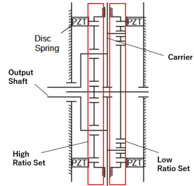
Figure 6 Gear sketch of the 2-speed planetary gear transmission
