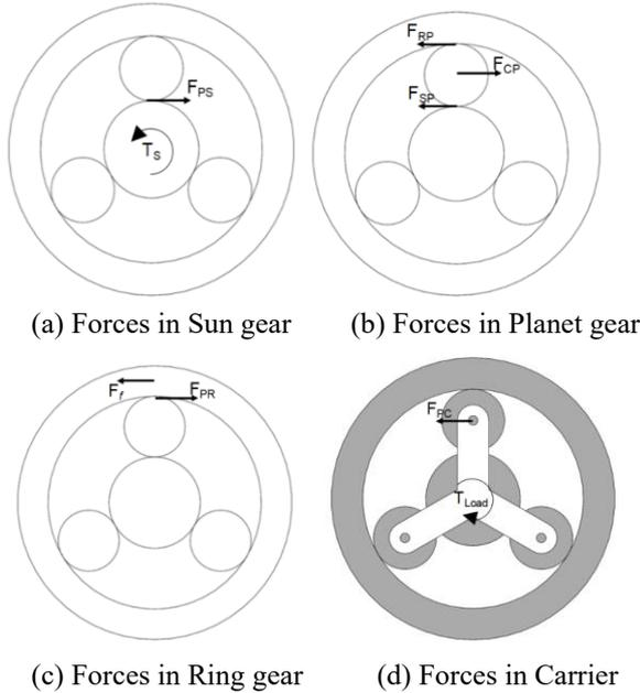
Figure 8 Forces between each components of a set of planetary gear set
