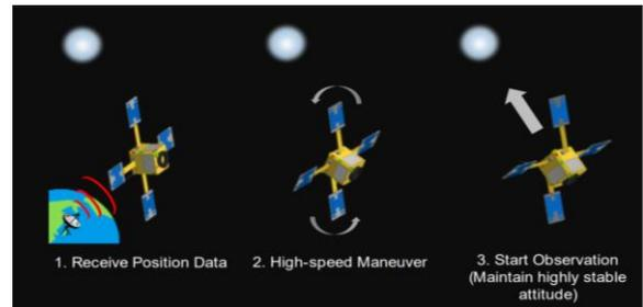
Figure 1 Procedure of VSAC system
