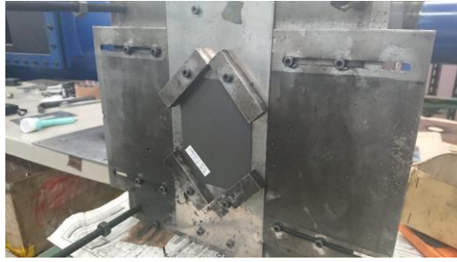
Fig. 1 Experimental setup for impact test 9)
