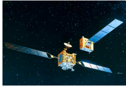
ETS-VII (1997) Rendezvous and docking technology demonstration
