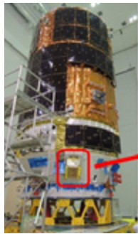
Space Debris Monitor on HTV-5 (image credit: JAXA)
