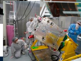
RCS (thruster) function test
