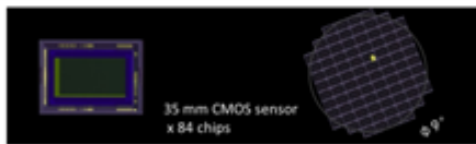
Array of 84 CMOS sensor covering FOV 9 o diameter credit: www.ioa.s.u-tokyo.ac.jp/tomoe
