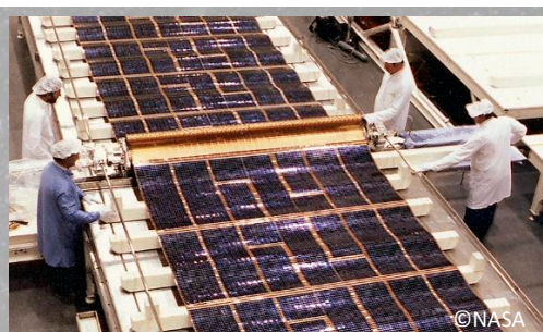
Replacement of SAP from Si to GaAs cells in Service Mission 3B (March 2002)
