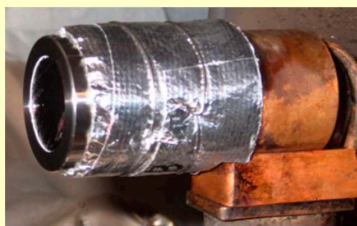
Test Configuration Specimen from Tank (CFRP/Aluminum Liner)
