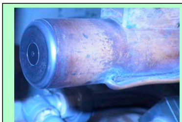
Probe of Facility Sensor: Gardon gauge
