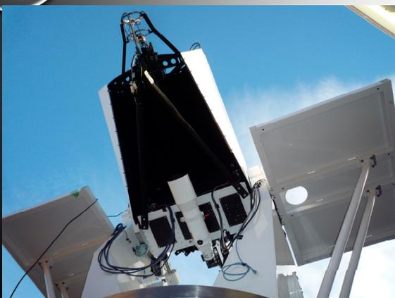
Light curve observations of 4 H-2A R/Bs are being carried out using 60cm telescope
