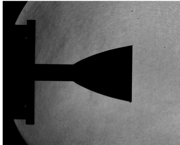
High enthalpy shock tunnel : HIEST Max enthalpy 25MJ/kg, Max stagnation pressure 150MPa, 0.5m test article
