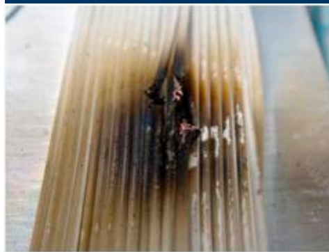
Impact-induced sustained discharge on power harness (ground experiment)
