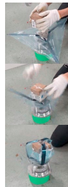
A prototype capture mechanism combined with a membrane. The gripper is activated when the target contacts the center of the gripper.
