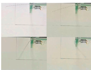
Motion of spring by high speed camera
