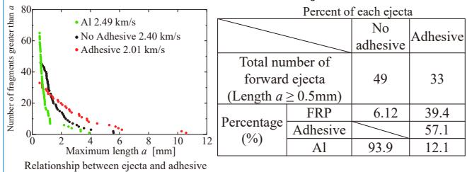
Total number of forward ejecta: Adhesive < No adhesive < Al (Length a ≥ 0.5mm)
