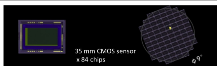
Array of 84 CMOS sensor covering FOV 9° diameter credit: www.ioa.s.u-tokyo.ac.jp/tomoe
