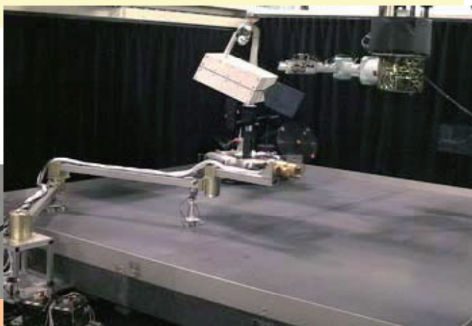
New joint mechanism & torque sensor
