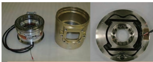
New joint mechanism & torque sensor
