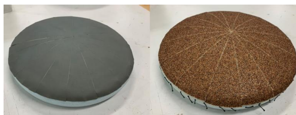
Fig.6 Surface of capsule provided roughness by sandpaper (Left#2000, Right: #40)
