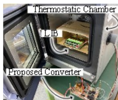
Fig. 6. Experimental platform using thermostatic chamber for LIB heating.
