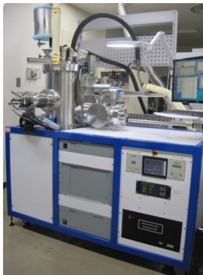
Fig. 3 The outgassing rate measurement apparatus.
