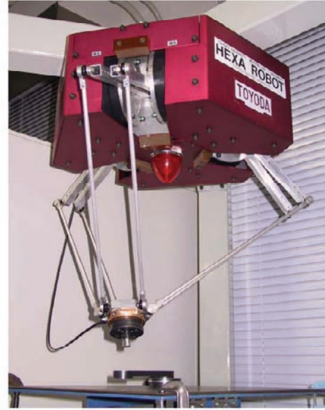
Fig. 2.2: Overview of a parallel robot HEXA
