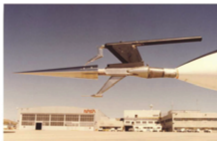
FIGURE 1.7 Transition cone flight experiment performed on a NASA F-15 aircraft at NASA Dryden Flight Research Center in the late 1970s. This was an example of a NASA aircraft adapted to conduct specific data collection for aerodynamic research. SOURCE: NASA Dryden Flight Research Center.
