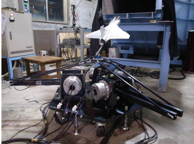
Achieved Roll Oscillation with amplitude of 10 deg and at frequency of 4Hz
