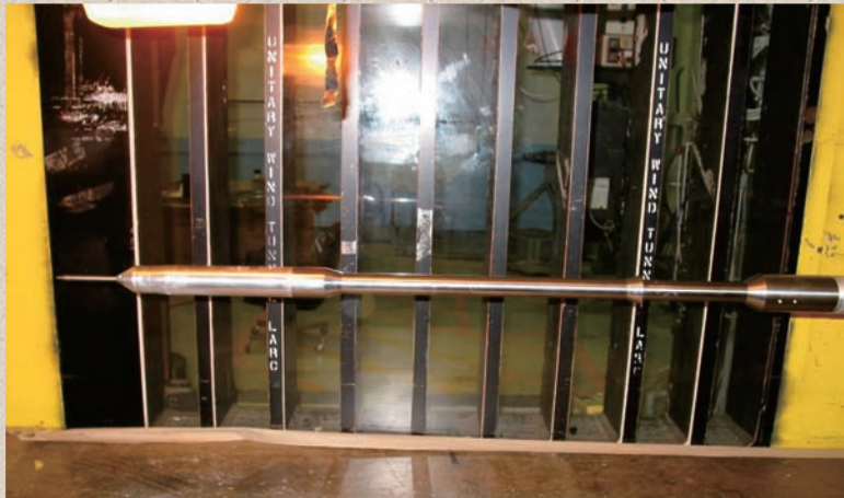
One-percent scale model of the Ares-like booster configuration in the NASA Langley Unitary Plan Wind Tunnel
