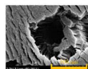
裏面反発 (V) D = 434 \mu\text{m} , v = 18 \text{ m/s}
