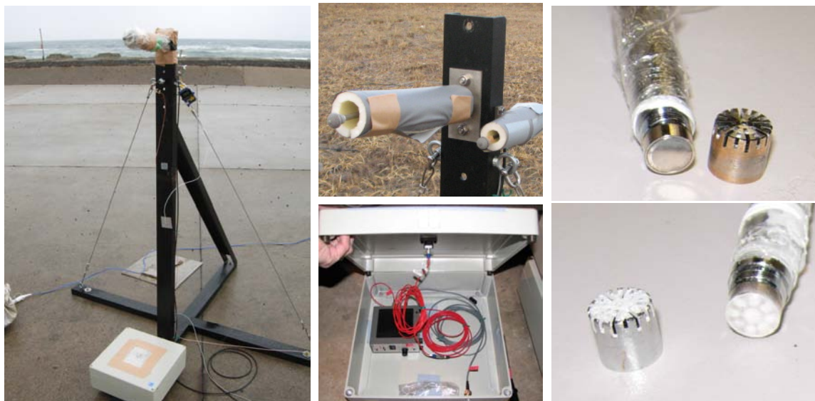
Fig.3-1. A microphone stand and a microphone box on the ground (left). A water-proof grid installed on the microphone (middle top), inside the box (middle bottom). Influence of Alumina particles (right top: normal, right bottom: contaminated).
