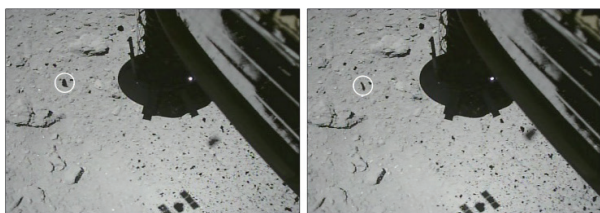
Figure 2. CAM-H images during the ascent of the spacecraft after the first touchdown. The particle in the white circle in the left image was spinning and moved from right to left and showed a flat shape in the image taken one second later (right).
