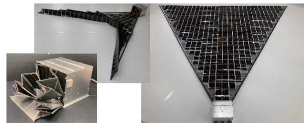
Figure 1. Thin-film solar cell paddle for small spacecraft to outer solar system
