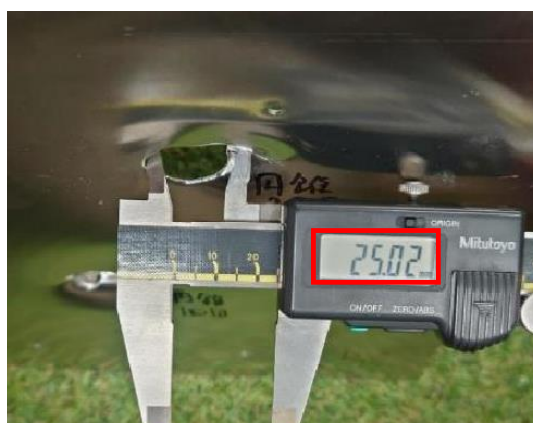
Penetration hole by non-rotating harpoon
