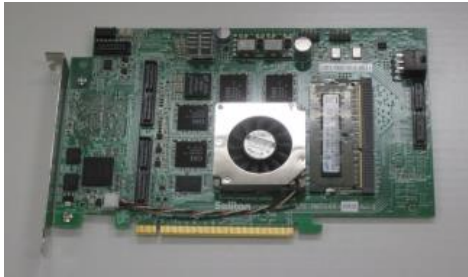
FPGA board, EXpresso A5 manufactured by soliton systems
