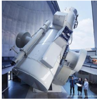
Kiso Schmidt telescope Wide-field telescope ( D_{\text{eff}} = 1.05 \text{ m} , f/3.1 ) (source: https://tomoe.mtk.ioa.s.u-tokyo.ac.jp/ )
