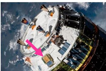
Fig.5 The space debris monitor on HTV<sup>4)</sup>
