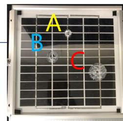
Fig.15 Solar array simulating impact marks
