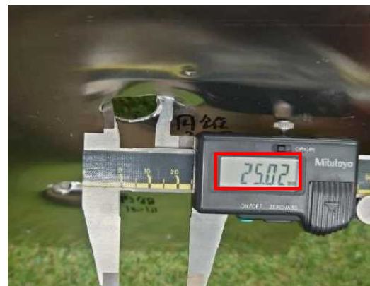
Penetration hole by non-rotating harpoon
