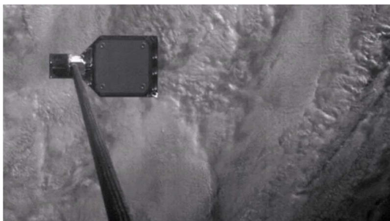
Shooting a deployable harpoon into a structure simulating space debris
