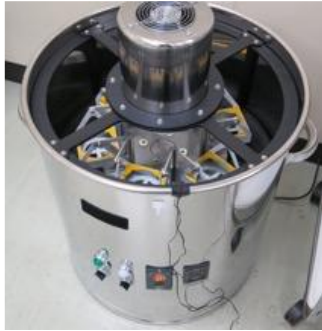
Fig. 1 Centrifuge MK3 generating hypergravity ~10G
