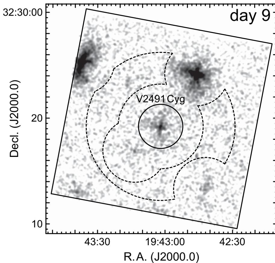
Fig. 1. Smoothed XIS image on day 9. Events recorded by the three CCDs in the 0.2–12.0 keV were used, excluding those in the 5.0–7.0 keV range to eliminate the signals from the calibration sources at the corners. The solid and the dashed circles indicate the source and background accumulation regions, respectively.
