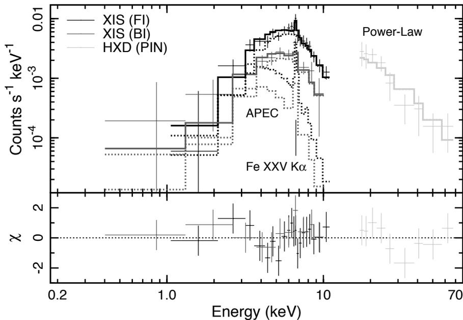
Fig. 2. Background-subtracted spectra and the best-fit model on day 9. The two XIS FI spectra with nearly identical responses were merged, while the BI spectrum was treated separately. The best-fit model is shown with thick lines (solid for total and dashed for each component) for FI, BI and PIN in different colors. The lower panel shows the residual from the best-fit model.
