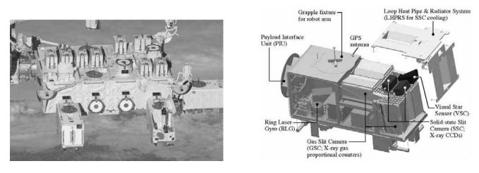
Fig. 1. MAXI in the orbit after installed on the station
