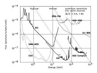
Fig. 4. Detection limits of the SXT-I/SXI and HXT/HXI for point sources.
