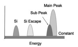
Fig. 3. Responses function of CCD, consists of 4 gaussian components and a constant component.
