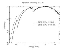
Fig. 2. Quantum efficiency of SSCU.
