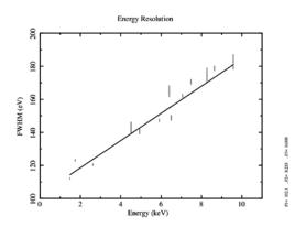
Fig. 1. The energy resolution of SSCU-Z CCD-0 and its fitted function.
