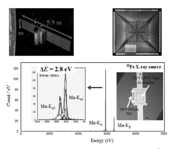
Fig. 1. Upper left: The DIOS spacecraft. Upper right: A picture of the 16×16 TES array. Lower left: Energy spectrum for <sup>55</sup>Fe X-ray source by a single pixel TES calorimeter. Lower right: the fabricated Ti/Au TES calorimeter with Au absorber.
