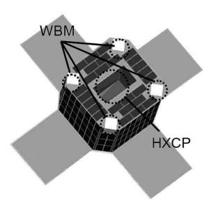
Fig. 1. TSUBAME configuration: Hard X-ray compton Polarimeter (HXCP) is centered at the observatory. Csl counters of the Wide-field Burst Monitor (WBM) are attached to each corner of the observatory.
