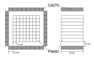
Fig. 2. Detector design for hard X-ray compton polarimeter (HXCP): Csl scintillators (absorber) surround plastic scintillators (scatterer).
