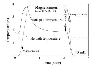
Fig. 3. Profiles of magnet current and temperatures
