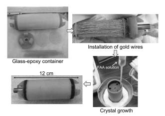
Fig. 1. Fabrication of FAA salt pill.
