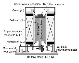
Fig. 2. Setup of the salt pill
