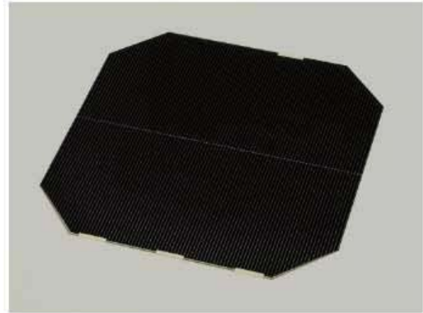
Fig. 9: Large area triple-junction space solar cell (8cm x 8cm with cropped corners) [7].
