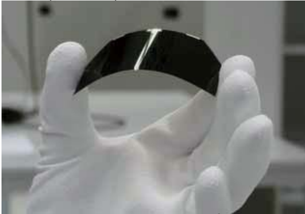
Fig. 7: Space solar cell ( A=30.18\text{ cm}^2 ) on 100 \mu\text{m} thin Ge substrate weighing 1.8 g. The weight reduction compared to 150 \mu\text{m} Ge substrates is 28% [7].
