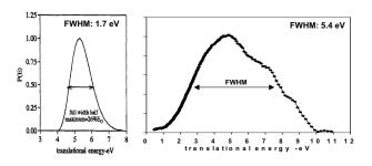
**Figure 2.** The energy distribution of atomic oxygen in low earth orbit space environment (left panel) and in laboratory simulated by a laser detonation source (right panel). Full-width at half-maximum (FWHM) is 1.7 eV and 5.4 eV for low earth orbit and for laboratory, respectively.
