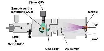
**Figure 1**. The laser detonation atomic oxygen beam source used in this study. Excimer and deuterium lamps are equipped as an external source of VUV.
