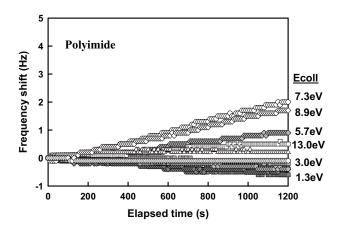
**Figure 4** Frequency shift of polyimide-coated QCM during atomic oxygen exposures with various collision energies. Average collision energies (Ecoll) in each exposure condition are shown in the right side of the panel.
