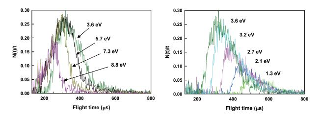
**Figure 3** Time-of-flight spectra of atomic oxygen beam (m/e=16) sliced by the high-speed chopper wheel. For better view of the each TOF spectrum, left and right panels show the TOF spectra in which slow-part and fast-part of the beam pulses are blocked by the chopper wheel. The same TOF spectrum (Ecoll=3.6 eV) is shown in both panels for comparison purpose.
