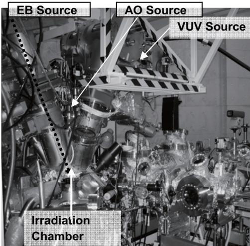
Fig. 2-1 Combined space effects test facility [1]
