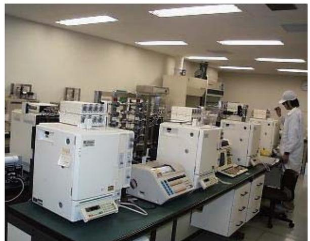
Fig. 5-2 Gas chromatography equipment for Test 7.
