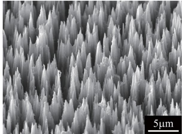
Fig. 2-2 Surface topographies of polyimide film [2].
