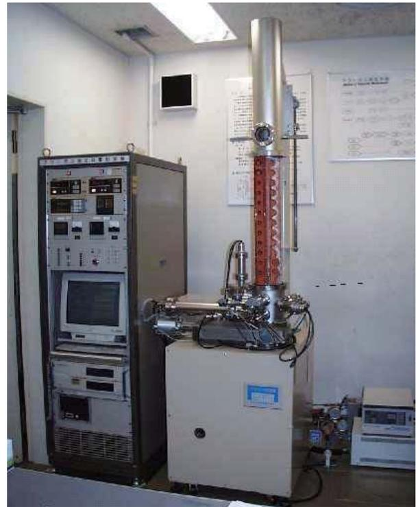
Fig. 2-4 Outgassing measuring system
