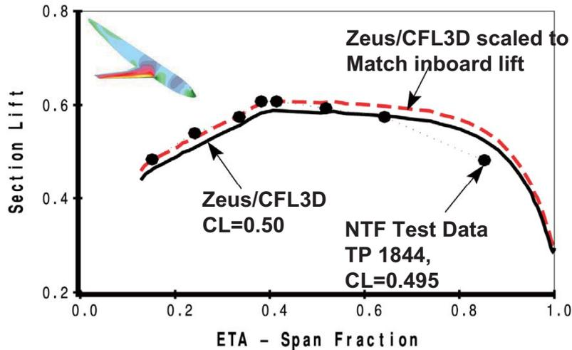
Increasing the nose down twist on the outboard part of the wing will result in a higher angle of attack when matching CL thereby better matching the wind tunnel force and pressure data.
