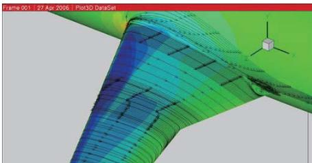
Overlay of Computed Streamlines, SST Turbulence Model, Re=5M
