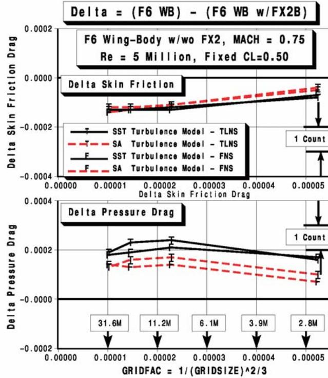
Drag increment variation is due to pressure drag changes we believe are related to the separation bubble prediction
