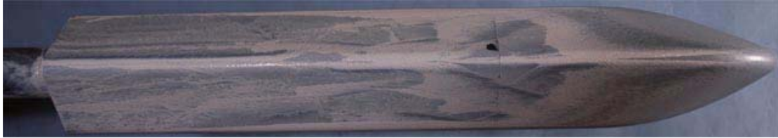
Oil Flow Visualization (M=4.0, AoA=30deg)
