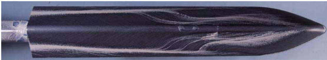
Oil Flow Visualization (M=0.3, AoA=30deg)
