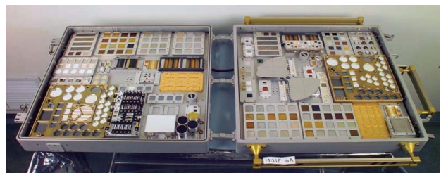
Fig. 4. Materials International Space Station Experiments (MISSE-6) pallet.
