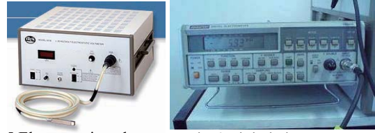
Fig.5 Electrostatic voltmeter Fig.6 Digital electrometer
