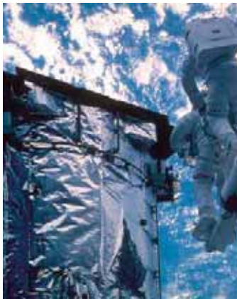
Fig. 3 Large cracks in HST MLI after 6.8 years in space.
