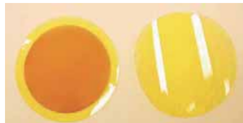
Fig. 15 TOR LM, 38.1 μm thickness post-flight (left) compared to a pristine control (right).
