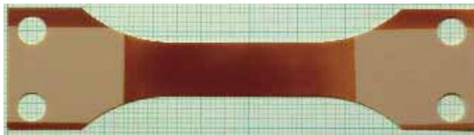
Fig.12 Surface appearance of the UV irradiated sample (34ESD ( 3.47 \times 10^4 J/cm 2 ), under 4.7MPa).
