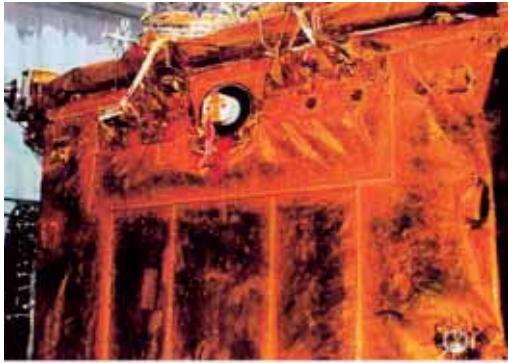
Figure 13 Discolored polyimide MLI surface of EPEX on SFU [5]
