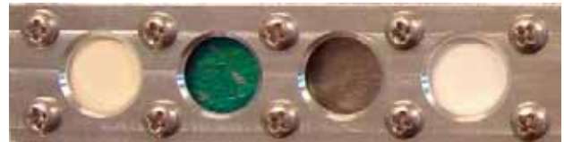
Fig. 26 Pre-flight photograph of one set of Cermet Coatings and Thermal Control Paints Experiment samples.
