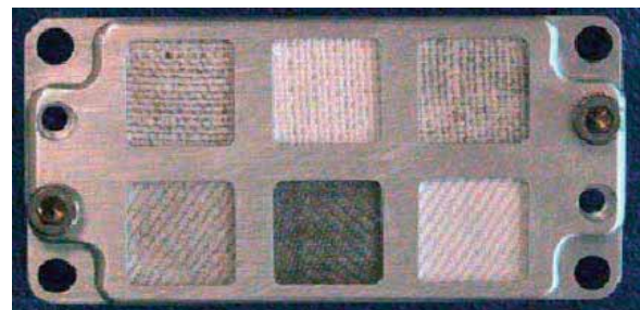
Fig. 40 Spacesuit Fabrics Exposure Experiment: the top row contains modern orthofabrics and the bottom row contains Apollo era \beta -cloth. The bottom middle sample is from Alan Bean’s Apollo 12 spacesuit left knee.
