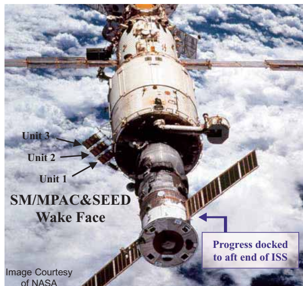
Fig. 2 SM/MPAC&SEED On-Orbit, Wake-Facing Side
